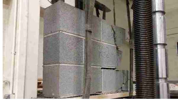
Figure C-9: Test Group 1 Masonry Panels E & F at Failure
