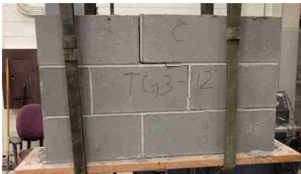
Figure C-13: Test Group 3 Masonry Panel C at Failure
