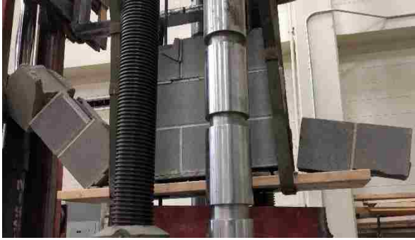
Figure C-9: Test Group 1 Masonry Panels E & F at Failure
