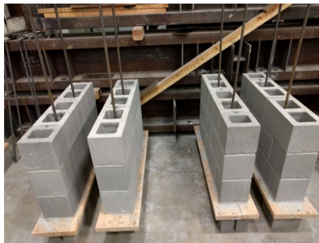
Figure 3-5: Panels Before Grouting
