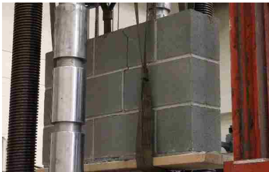
Figure C-8: Test Group 1 Masonry Panels C & D at Failure
