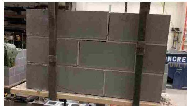
Figure C-13: Test Group 3 Masonry Panel C at Failure
