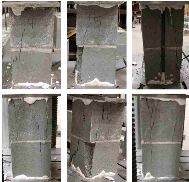
Figure C-6: Masonry Prisms at 28-Day Failure
