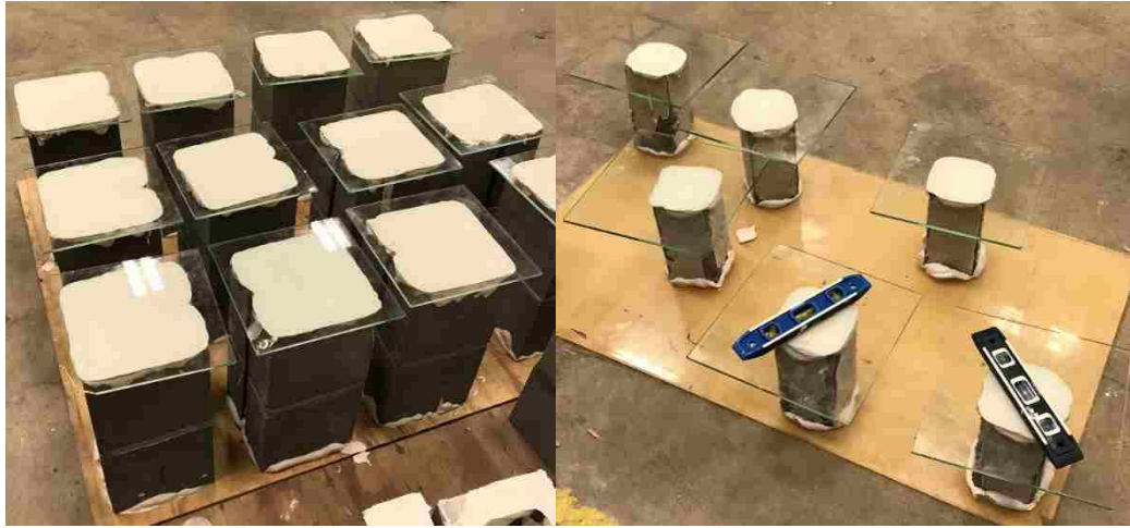
Figure 3-13: Masonry and Grout Prism Capping
