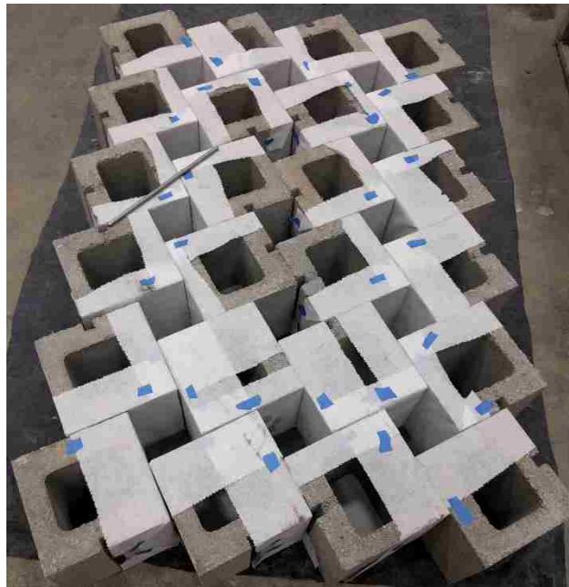
Figure 3-1: Grout Prism Molds
