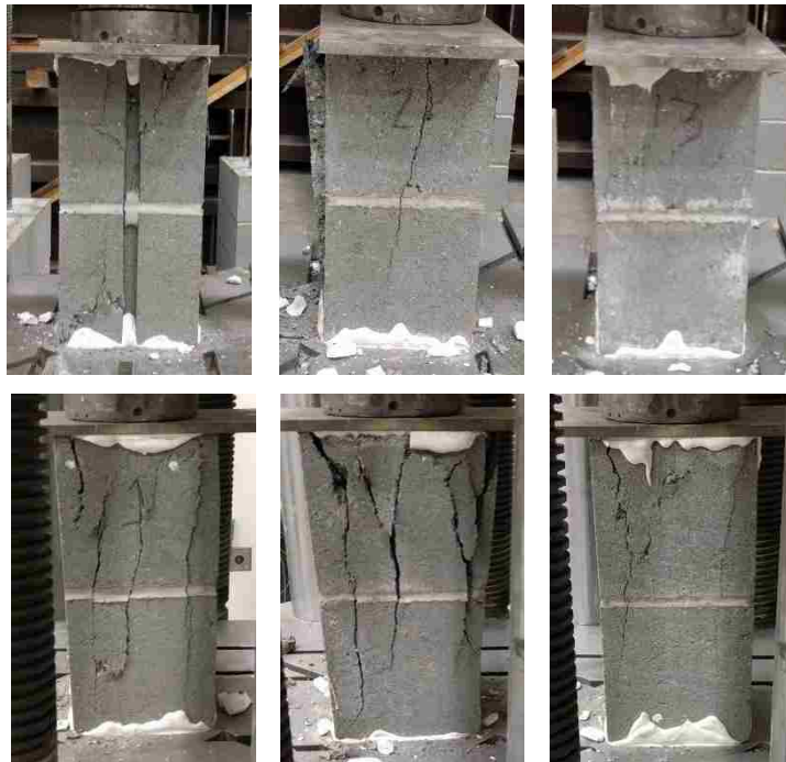
Figure C-4: SCG Prisms at 32-Day Failure
