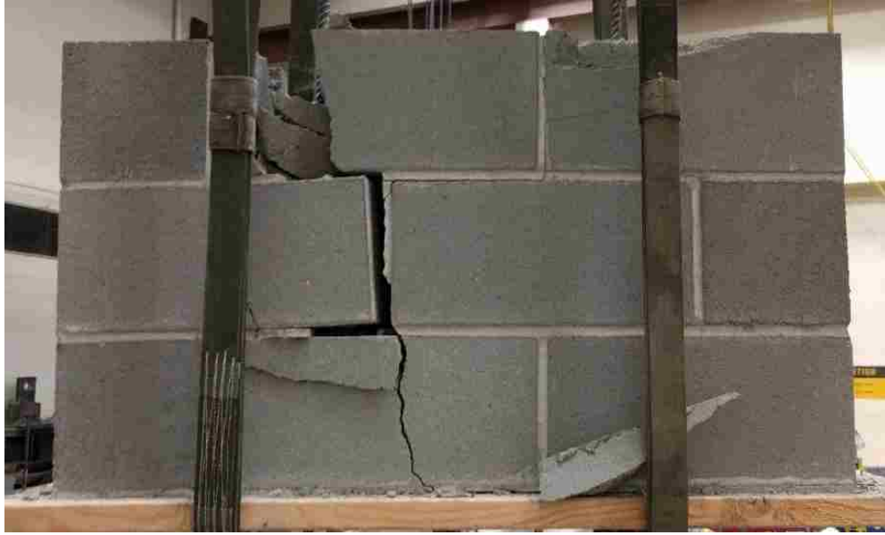
Figure 4-7: Typical Masonry Panel After Failure
